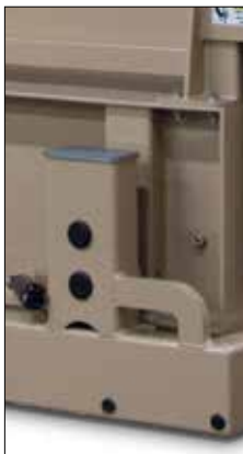
Load cell enclosure
